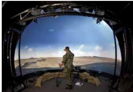
A total of thirteen F22 series projectors are blended into a single image in a military simulation projector. The F22 series, thanks to its small size, and flexible lens configurations, is perfect for this type of application, and reduces complexity and real estate requirements to a minimum. Images courtesy of Air Force Research Lab (AFRL) Mesa, AZ, USA.
